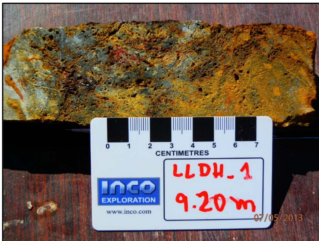
Figure 1 – Hole LLDH_1 core sample at 9.20m showing extensive sulphides in vuggy quartz vein
