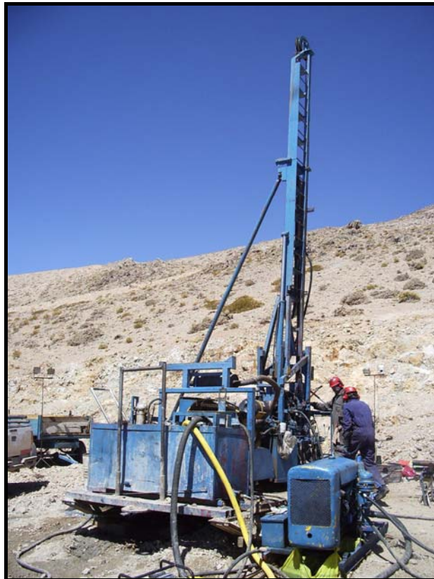
Figure 6 – Phase 2 Program diamond drilling rig established on MC-4 drill site
