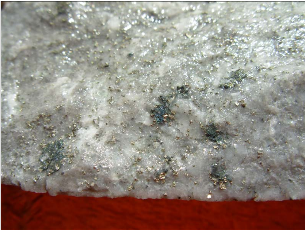
Figure 1 - MC-1_53-59m core detail: Disseminated pyrite, chalcopyrite and bornite in potassic-altered and silica-flooded diorite porphyry breccia.
