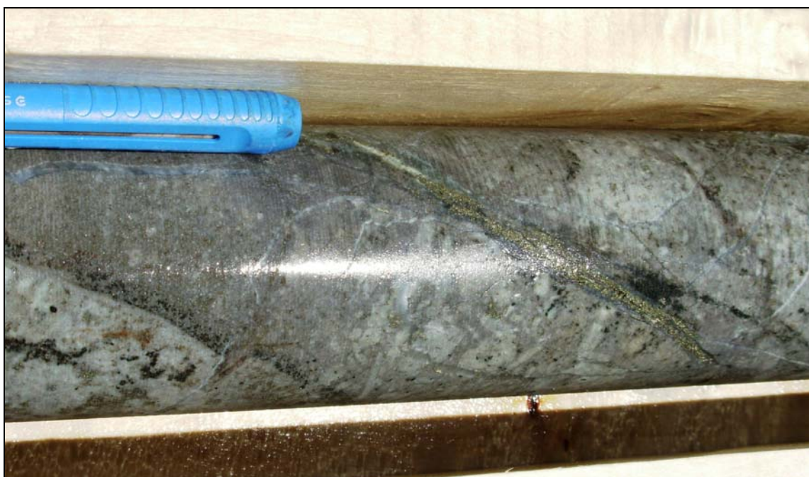
Figure 3 - MC-3_217.5m core detail: Pyrite and chalcopyrite in stock-work of gypsum veinlets and disseminated throughout sub-angular diorite porphyry breccia (15% total sulphides). Potassic alteration with silicification.
