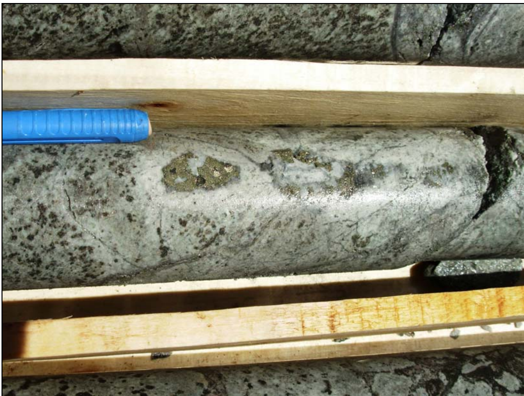
Figure 2 - MC-1_307m core detail: Breccia matrix veinlets of gypsum, pyrite, chalcopyrite, magnetite and chalcocite in strongly potassic-altered diorite porphyry breccia.
