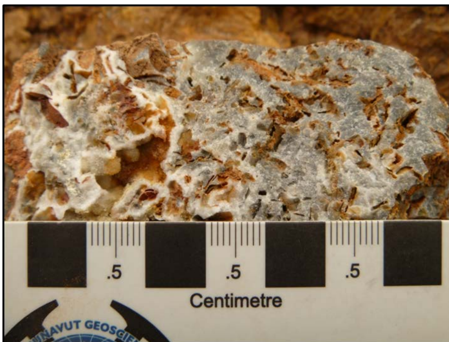
Plate 4 - Hand Specimen of the quartz reef showing typical epithermal-style characteristics
