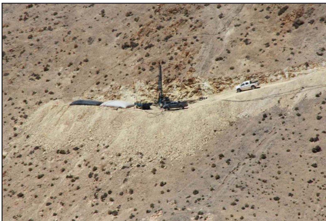
Figure 3 – Drill site DDH MC-2 showing oxidised & mineralised structures exposed in road cutting.
