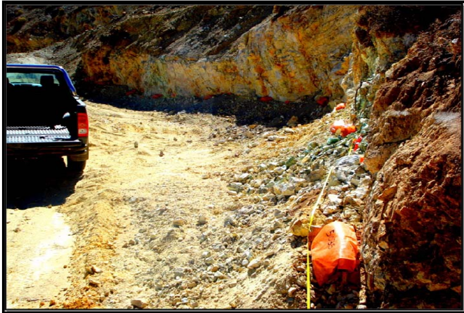
Figure 5 - Drillhole MC-4 drill pad cutting showing jarositic clays, limonite, copper oxide and other features typical of a porphyry copper leached cap
