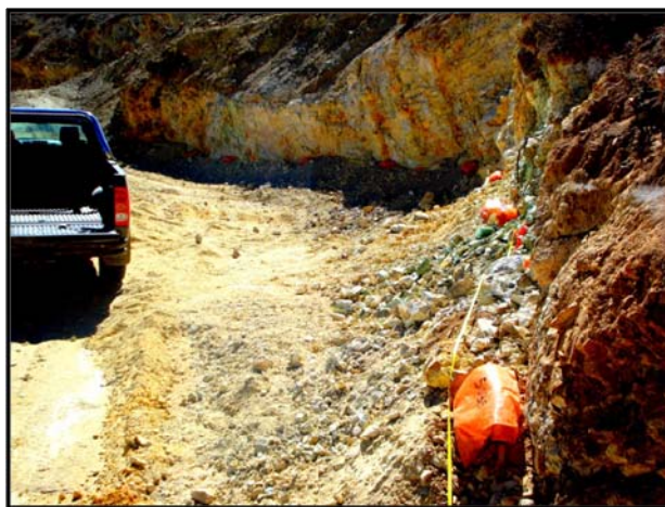
Photograph 2 - Part of MC-4 drill pad excavation showing intense yellow clays (jarosite) and distinct bands of brown limonite which may represent original sulphide-rich zones
