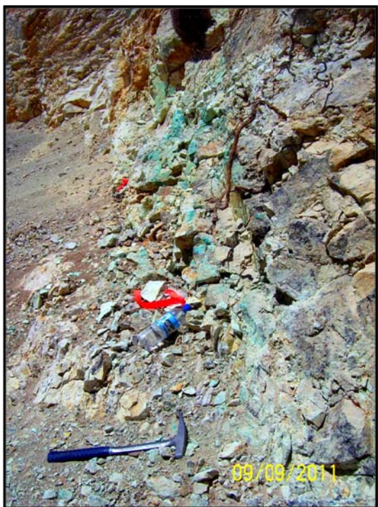
Photograph 1 - Detail of wall in MC-4 drill pad excavation showing bands of copper oxides (green-blue) and a manganese-rich mineral (black)
